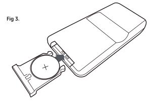
As the battery becomes exhausted the operating distance will shorten. When the remote no longer operates the unit, replace the battery with a new CR2025 lithium battery. (Fig 3)
