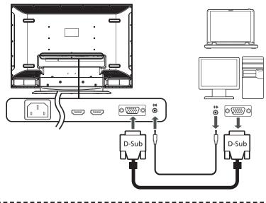
For VGA input, Acer recommends setting your PC's external monitor resolution to 1366 x 768 pixels @ 60 Hz refresh rate.
