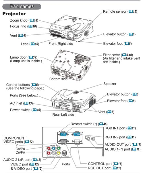
**NOTE** (\*) About Restart switch: This projector is controlled by an internal microprocessor. Under certain exceptional circumstances, the projector may not operate correctly and the microprocessor will need to be reset. In such a case, please push the Restart switch by using a cocktail stick or similar, and before turning on again, make the projector cool down at least 10 minutes without operating. Only push the Restart switch in these exceptional instances.
